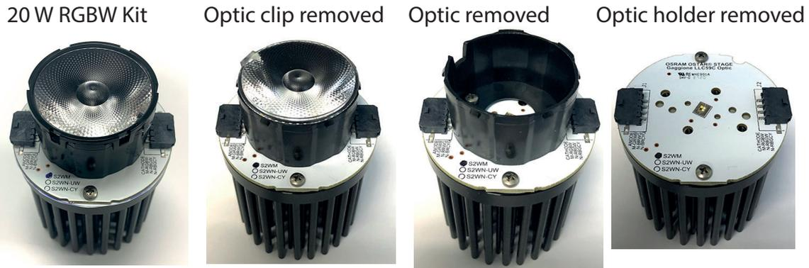
To mount the new optic and holder, simply place the new holder on top of the light engine and find the corresponding alignment and screw holes. Screw the holder into the light engine in the two available holes and then snap the optic into place within the holder. The holder is keyed so that optic can only go in one way. Figure 18 shows the mounting of the new optic and holder.
