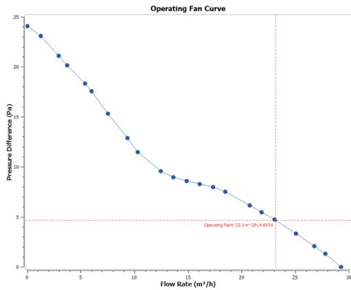
Figure 14: Thermal simulation results 40 W RGBW kit with fan
