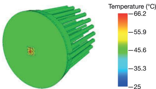
You can observe that the resultant junction temperature is ~15 °C cooler than the design with the thermal interface material. You can also observe that the heatsink temperature is hotter in the second simulation; this is an indication that the heat is moving into and out of the heat sink in a more efficient manner than in the first simulation.
