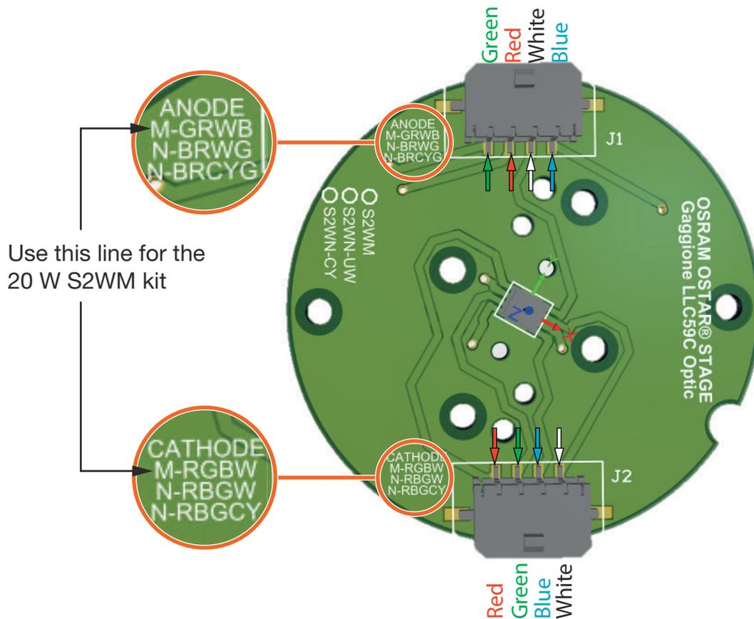
The kit comes with wire harnesses; however, all the wires are black and are not color coded. Therefore, you need to take care to identify which wire is connected to which pin on the PCB assembly before connecting to your power supply or driver electronics.
