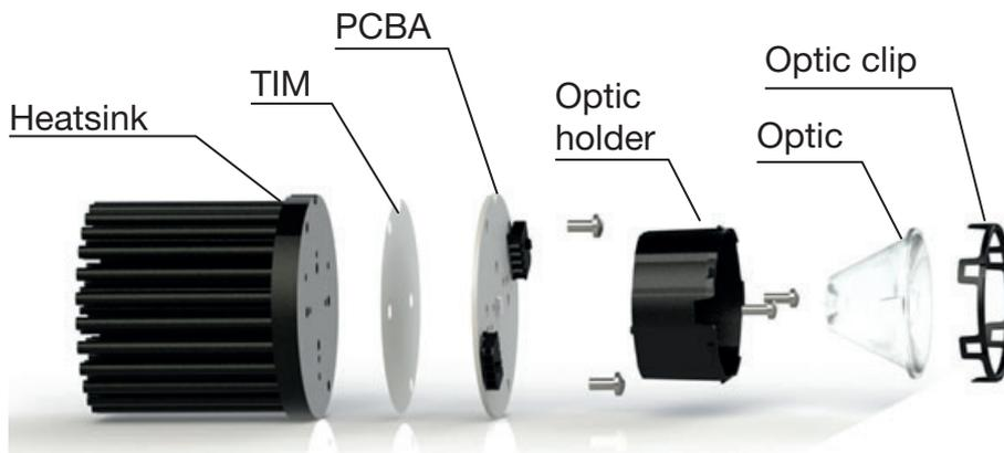
An exploded view of the light engine of the 40W RGBW and 40W RGWA variants is shown in Figure 3.
