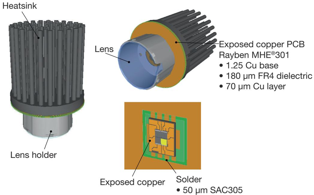
The simulation results show that the resultant LED junction temperature is under the rated maximum junction temperature of the LED. This means that you can operate all 4 die at 2 A simultaneously in a room temperature environment with no concerns related to heat. The results are shown in Figure 11
